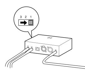
The last step in the process is to set the "1-2-3" switch on the side of the IF6P to "1."
